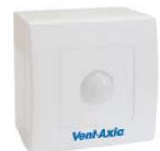
Fits any UK single gang mounting box. Adjustable timer overrun (5-25 minutes). Range of detection up to 10 metres. Designed to meet IP43. Ambient operating temperature range 0°C to +50°C. Supply voltage 24V DC SELV.
