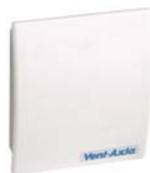
24V DC SELV. 0 - 2000ppm CO<sub>2</sub> working range. 0 - 50°C working range. Auto-calibrating NDIR CO<sub>2</sub> absorption sensor. Thin film platinum temperature sensor for high accuracy. Dimensions:100 x 84 x 25mm (H x W x D).
