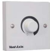
Manual control. Located remotely. 24V DC SELV. Ambient operating temperature -5°C to +40°C. Dimensions:84 x 84 x 30mm (H x W x D). Will fit single gang box for surface mounting.
