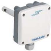
24V DC SELV. 0 - 2000ppm CO<sub>2</sub> working range. Auto-calibrating NDIR absorption sensor. Stable drift compensation. Adjustable probe length. MAX. IP Rating 65.
