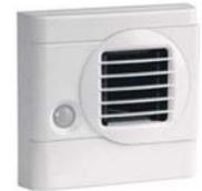
12V AC SELV unit using the main transformer unit supplied. Integral PIR person presence sensor controlling damper. Auto-humidity control damper response at all times. 100° viewing angle. Temperature range 0 - 50°C .Size: 158 x 150 x 35mm (H x W x D). MAX airflow 70m<sup>3</sup>/hr @100 Pa.
