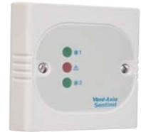
24V DC SELV. Directly connects into the SCU. Used for single and twin fan mounting. Ambient operating temperature -5°C to +50°C. Dimensions:86 x 86 x 28mm (H x W x D).
