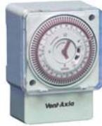
The 7 Day TimeSwitch gives twelve On or Off positions per day and can be set for 7 days. The cycle will repeat until changed. Volt free switch connection to Sentinel.
