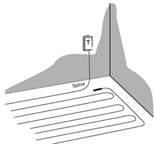
**2.** Avoid stepping or dropping items on the cable and use caution in further works with pouring the floor.
