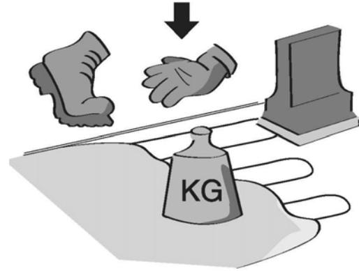
**7.** The heating cable is not to be used before the concrete/screed/mortar has naturally hardened and dried. This can take up to 6-8 weeks. Please consult the instructions/guide provided by the vendor of the concrete/screed/mortar.
