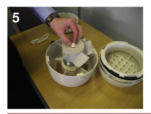
You should normally be able to unscrew the impeller nut by hand, however if it has siezed up you can use a suitably sized flat head screwdriver
