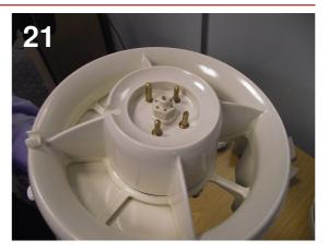
Whilst holding the motor into place, turn the housing over and refit the motor nut using a suitable tool to tighten it
