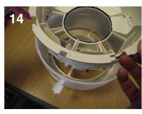
Place the shutter assembly into the fan housing as shown with the word "BASE" towards the retaining screw at the 6 o'clock position
