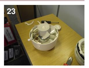
Flip the fan housing over and before refitting the impeller, ensure you have the 3-part washer set in place or refit on the motor shaft/spindle in the following order - metal flat washer, rubber flat washer, metal cone washer, then you can fit the impeller followed by the impeller nut.
