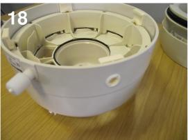
Ensure that the two retaining clip caps with the holes are re-fitted towards the base of the housing one either side of the retaining screw at the base (6 o'clock position) of the housing as you will then need to pass the pull-cords (where used) from the shutter assembly through these holes remembering to have crossed the cords over before placing through the retaining clip holes. [Note - we have not fitted the shutter pull cord in this exercise.
