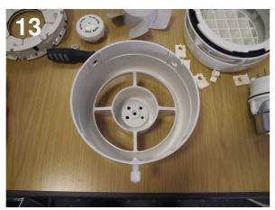
Next place the fan housing with the retaining screw at the base (6 o'clock position)
