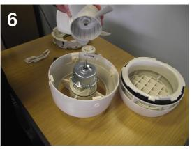
You should now be able to lift off the impeller to reveal the motor
