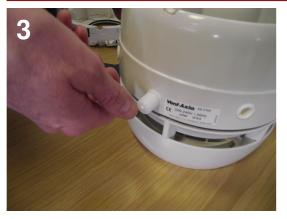
Unscrew the retaining screw at the base of the fan and then remove the fan/housing assembly from the external grille
