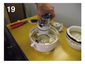
Carefully replace the motor back into the fan housing. The positioning of the motor connection pins will only allow the motor to fit properly in the one position
