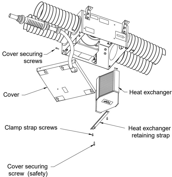
In addition to removing odours, providing fresh air and removing heat, this unit extracts airborne impurities such as dust, dirt and grease. These gradually build up and detract from the efficiency and appearance of the unit.
