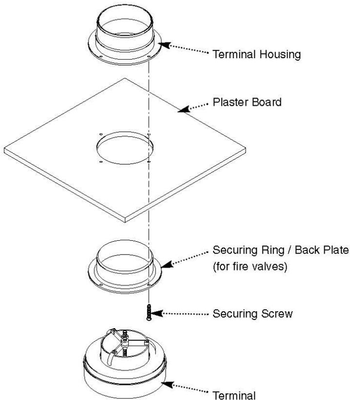
8. A shell bit is recommended for drilling holes in the ceiling to accommodate the housings for supply and extract air terminals (SV100 and EV100). Make sure that the drilled area is clear of structural members, water and gas pipes or electrical cables and that there is enough clearance behind the ceiling board for duct access and securing ring. Ceiling terminals should preferably be fitted equidistant from adjacent walls, be mindful that coving may be subsequently fitted.
