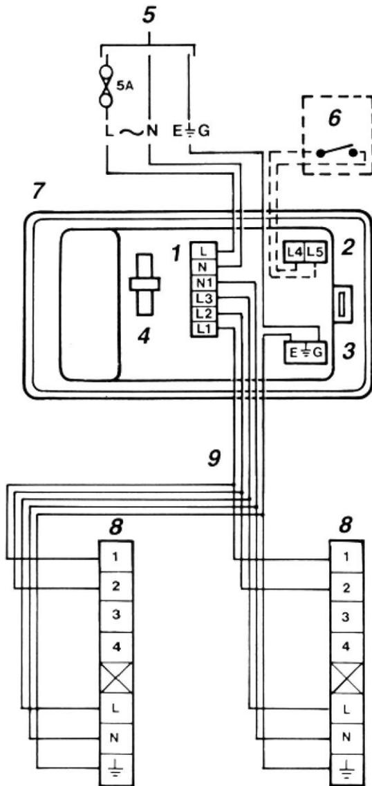
Current heat recovery ventilation unit terminal blocks as fitted to HR500 MKIII and HR500X units
