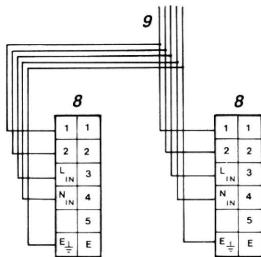
Earlier heat recovery ventilation unit terminal blocks as fitted to HR500 MKI and MKII units
