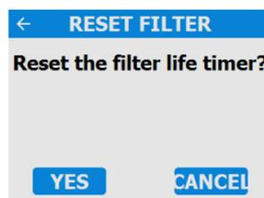
5. After maintenance of the filters, the filter timer can be reset by going to Settings/Reset filter.
