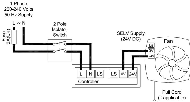
**Fig 10.** Wiring diagram with LS connection.
